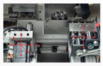
Thanks to the new design and to the use of two completely independent cross tables for the front and back machining units, the NM6 Flexi breaks the limits of flexibility and performance. Two parts can be manufactured at the same time: one part machined in the turning and front machining unit while the second part positioned in the counter spindle is undergoing back and side operations.
