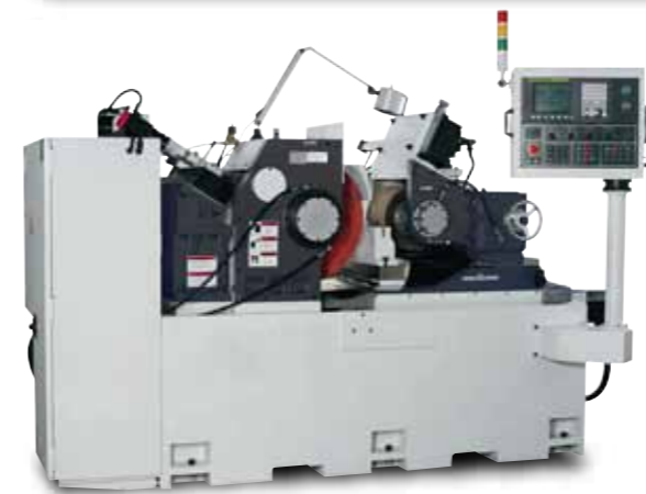
5 AXIS X1, Y1 axis regulating wheel dressing w/ interpolation. X axis grinding wheel dressing. Z axis regulating wheel lower slide movement. Z1 axis regulating wheel upper slide movement.
